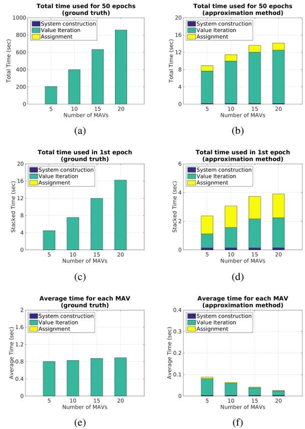
Fig. 7. Time performance comparisons (data from fifty trials). (a)(b) Total time used for computing 50 epochs for the ground truth and the approximation method, respectively; (c)(d) The time used for computing the first epoch (the most expensive epoch); (e)(f) Average time for each MAV in the two methods.
