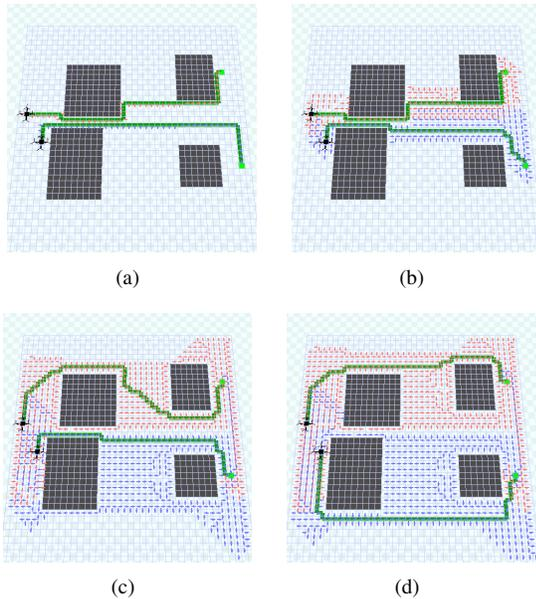
Fig. 6. Two MAVs refine policies locally. (a) Deterministic MSMG paths; (b)(c) As local spaces are exploited, the policies (and expected paths) are improved to avoid obstacles and narrow spaces; (c) Final refined policies and expected trajectories within the decomposed subspaces.
