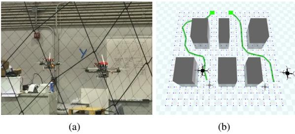
Fig. 5. Experimental demonstration. (a) A miniature multi-MAV system with two micro air vehicles whose states are fully observed by a motion capture system; (b) Visualization of physical experiments where two MAVs navigate to two goals (green grids) among a group of obstacles (black blocks). Expected trajectories are planned across the safest regions.
