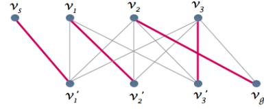
Fig. 3. Bipartite graph illustrating trajectory generation for one agent, where  $V = \{v_1, v_2, v_3\}$ ,  $V' = \{v'_1, v'_2, v'_3\}$ ,  $V_s = \{v_s\}$ ,  $V_g = \{v_g\}$ . Matched edges are in red bold, others are unmatched edges; goal trajectory  $v_s - v_1 - v_2 - v_g$  in  $G^d = (V, E)$  is obtained from the augmenting path  $v_s - v'_1 - v_1 - v'_2 - v_2 - v_g$  in the matching graph  $\tilde{G} = (V, V', \tilde{E})$ .
