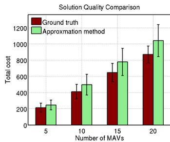
Fig. 8. Comparison of solution quality reveals limited sacrifice of optimality given the approximation method.
