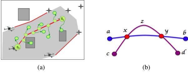
Fig. 4. (a) Local states fringing. Red lines are MSMG paths connecting to goals (stars). The green circles are fringe states and the shaded area represents local state space for the bottom-left MAV; (b) If path  $a \rightarrow b$  is locally optimal, the refined path  $c \rightarrow d$  will not cross path  $a \rightarrow b$ . Otherwise, it contradicts the local optimality assumption of path  $a \rightarrow b$  and its segment  $x \rightarrow y$ .
